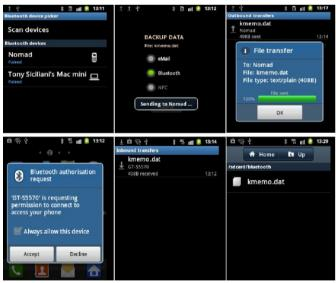
Note that, once the receiver accepts the connection. the received file (*kmemo.dat*) is saved inside the BT folder on the SD card. All the lower-level data transfer has been handled by the Android OS.
