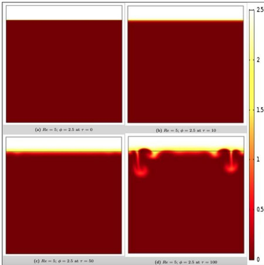
**Fig. 2: Evolution of temperature field in convective flow for  $Re = 5$ ,  $Fr = 2.5$  and Prandtl number  $Pr = 9.5$  and dimensionless temperature  $\phi = 2.5$  at the upper section within the time range  $0 \leq \tau \leq 100$ .**
