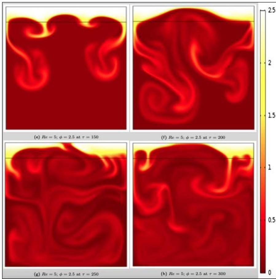
**Fig. 3:** Evolution of temperature field in convective flow for  $Re = 5$ ,  $Fr = 2.5$  and Prandtl number  $Pr = 9.5$  and dimensionless temperature  $\phi = 2.5$  at the upper section within the time range  $150 \leq \tau \leq 300$ .
