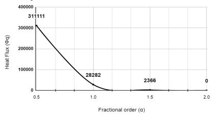
Figure 2.1:Heat Flux v/s Fractional order on concrete wall
